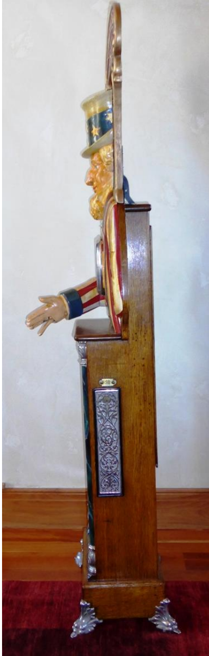
Fig. 14: Side view shows the fancy cast cash box cover. The cast feet have a hole in their tips so that the machine can be anchored to the floor, probably due to the top-heaviness with metal castings on top and wood base – and anticipating users being aggressive with the hand shake to get to 300 and the bell ring!
