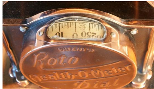
Health-O-Meter original Model 100 bath scale with drum-type dial
