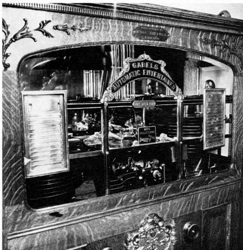
Photo 7. Close up of the front window. The tune card holders hang on each side, the coin counter is visible below the "Make Selection There" sign and the needle magazine is shown upright in the center. The tag above says "Pat. Apld. For".
